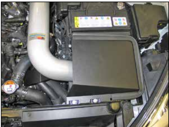
27. Install the cover onto the heat shield and then secure it to the heat shield and core support with the hardware provided. NOTE: the cover tab should slip in-between the heat shield and edge trim before securing.
