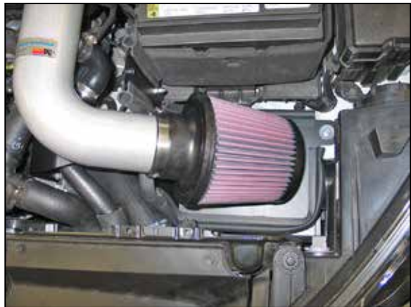
25. Install the K&N® air filter and secure with the provided hose clamp. NOTE: Drycharger® air filter wrap; part # RX-4990DK is available to purchase separately. To learn more about Drycharger® filter wraps or look up color availability please visit http://www.knfilters.com ®.
