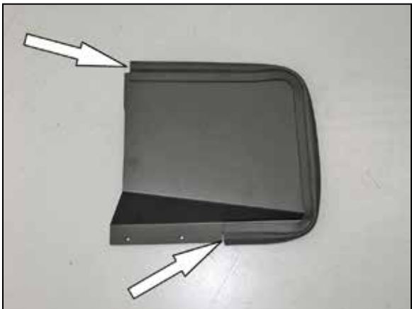
26. Install the 21”long section of edge trim onto the heat shield cover as shown.
