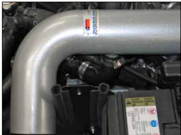
23. Feed the air injection hose assembly under the tube and mounting bracket and then connect the Open end of the air injection hose to the K&N® intake tube and secure with the provided hose clamp.
