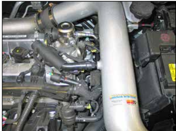
24. Reconnect the crank case vent hose and secure with the factory spring clamp.
