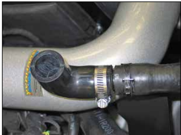
22. Connect the 90° air injection hose to the factory injection hose as shown and secure with the provided hose clamp.
